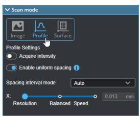
5. Capture a profile to make sure the target is in the sensor's field of view.
