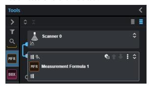
3. In the **Inputs** section, set the Measurement Formula's **Variable 1** input to the output of the measurement you need to scale.
