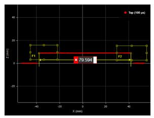
8. Set Feature 1 to MinX and Feature 2 to Max X, enable the Width measurement output.
