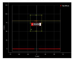
8. Set the feature to Average and enable the Z measurement.
